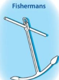
Awkward to stow and heavier than other anchors of similar holding power.
