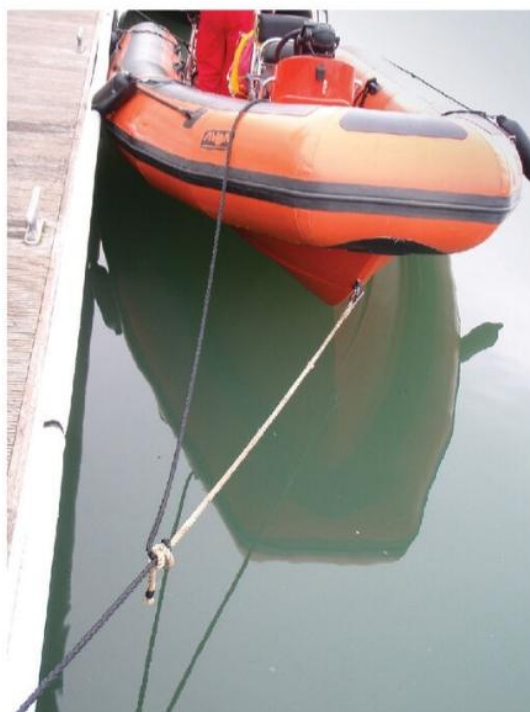
The black line is the anchor line. The white line is the bow line and is tied to the anchor line. The load of the anchor is transferred to the bow line through the knot.
